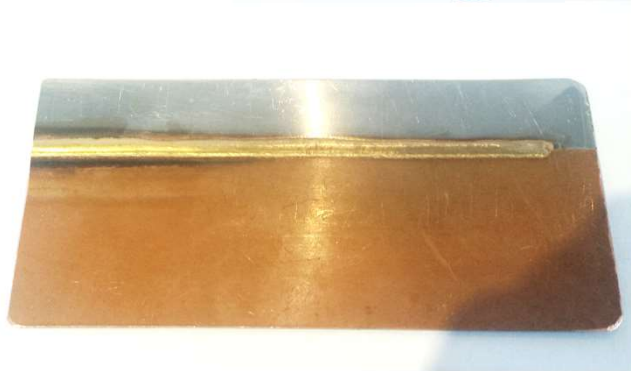
Direct welding of stainless steel caps on copper body with CMT welding . ( Mig-Mag welder)
