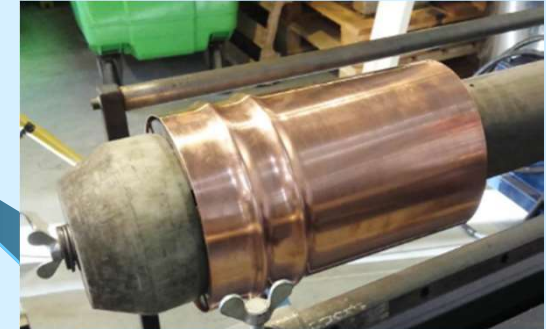
Production of copper tank 0,8 mm with 0,12 mm SSL coated copper layer.
